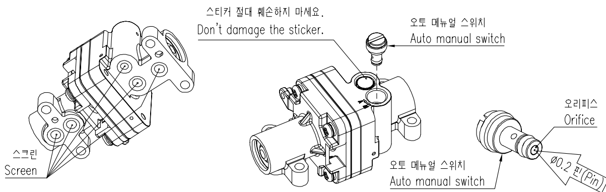
Fig. 8-1: Pilot unit and Auto manual switch
